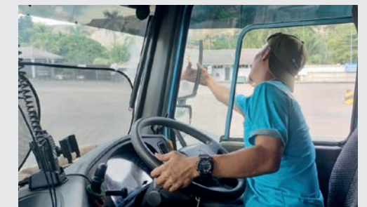
A participant practising the correct method to adjust rear view mirrors to minimise blind spots.
